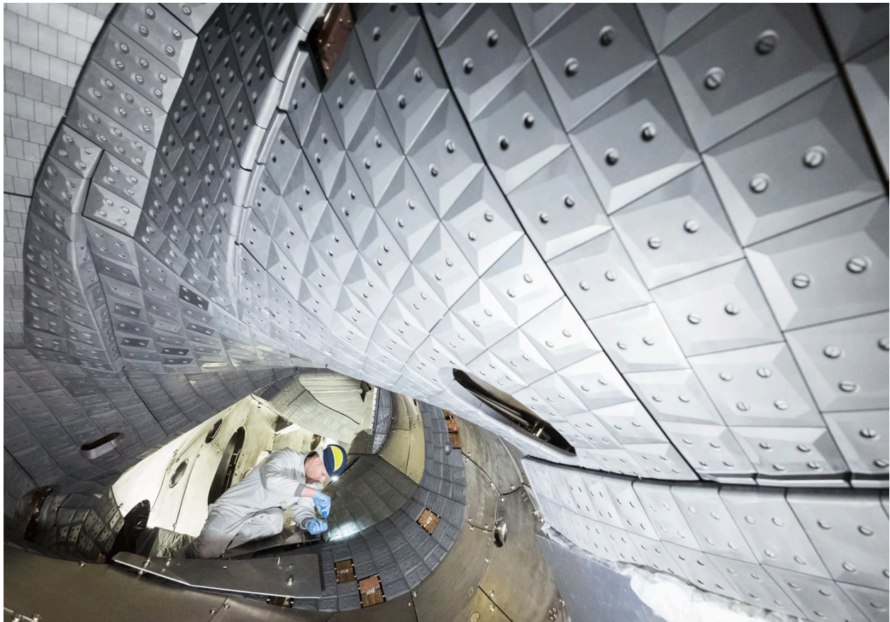
Figure IV.1-1. International facilities such as W7-X (pictured here) provide opportunities for testing novel plasma configurations and conditions not accessible by domestic facilities. Shown here is a view inside the W7-X plasma vessel with graphite tile cladding. Photo: MPI für Plasmaphysik, Jan Michael Hosan [from article “Wendelstein 7-X achieves world record” (June 25, 2018), https://www.ipp.mpg.de/4413312/04_18 ]
