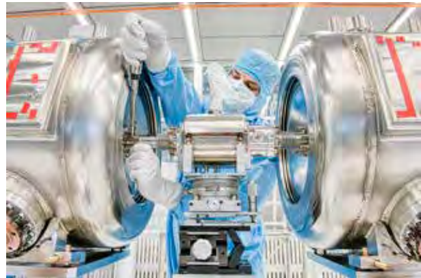
Fig. 3.3. A technician works on a 325-megahertz spoke resonator cavity string in one of the cleanrooms at Fermi National Accelerator Laboratory. The device is part an accelerator upgrade project that will improve the lab's accelerator complex and the beam it provides to experiments. [Courtesy Fermilab]
