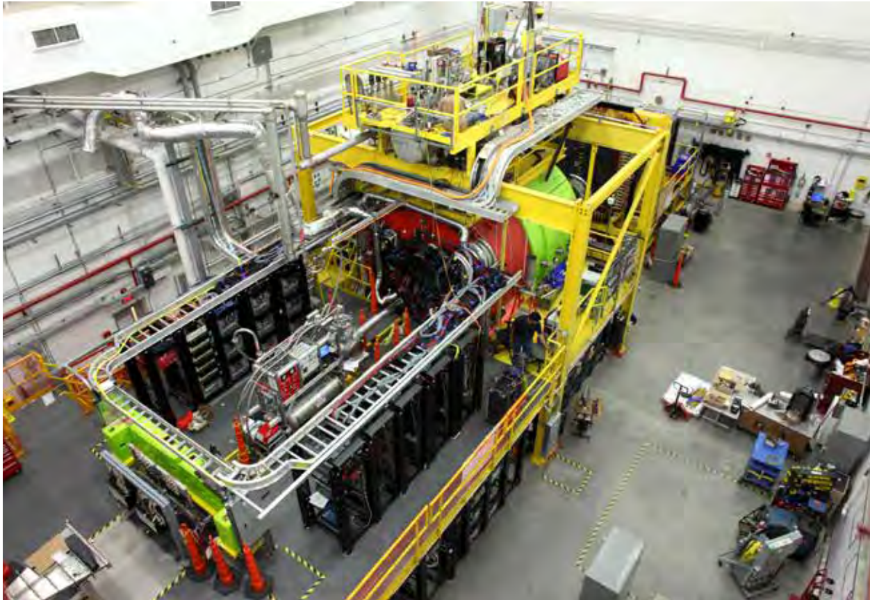
Fig. 2.1. Experimental Hall D at the Continuous Electron Beam Accelerator Facility is dedicated to the operation of a large-acceptance detector for experiments with a broadband, linearly polarized photon beam produced by \sim 12 GeV electrons. [Courtesy Thomas Jefferson National Accelerator Facility]
