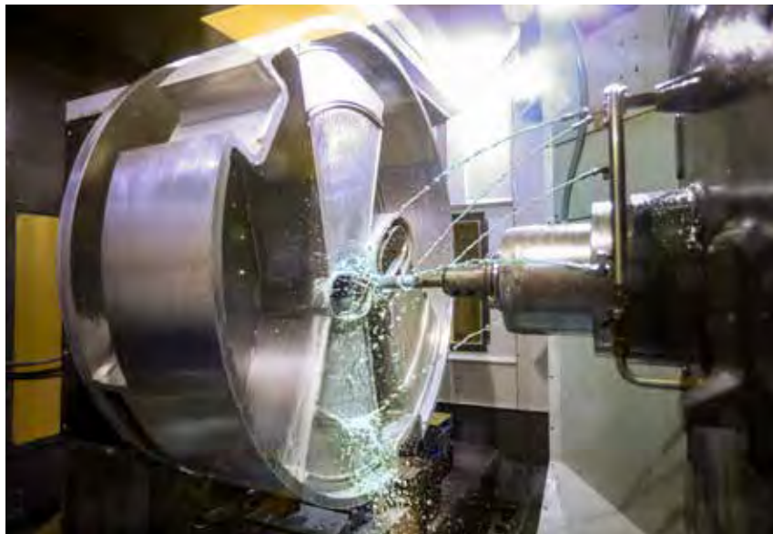
Machining cadmium for the Inner Reflector Plug at the Spallation Neutron Source. [Courtesy Oak Ridge National Laboratory]
