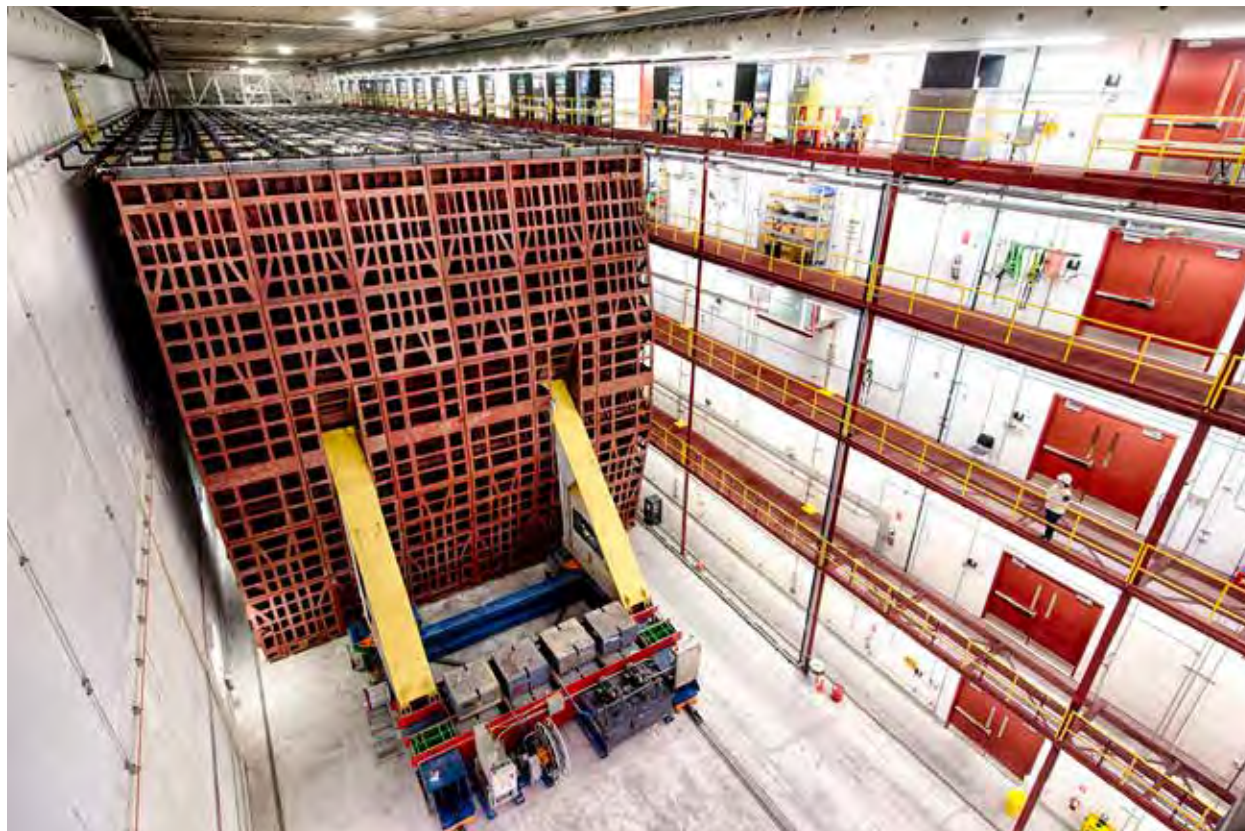
Fig. 2.2. The enormous NOvA far detector in Ash River, Minnesota, sits in the path of Fermi National Accelerator Laboratory's intense neutrino beam and captures particle interactions. Researchers use this data to better understand how the subatomic world works. [Courtesy Fermilab]
