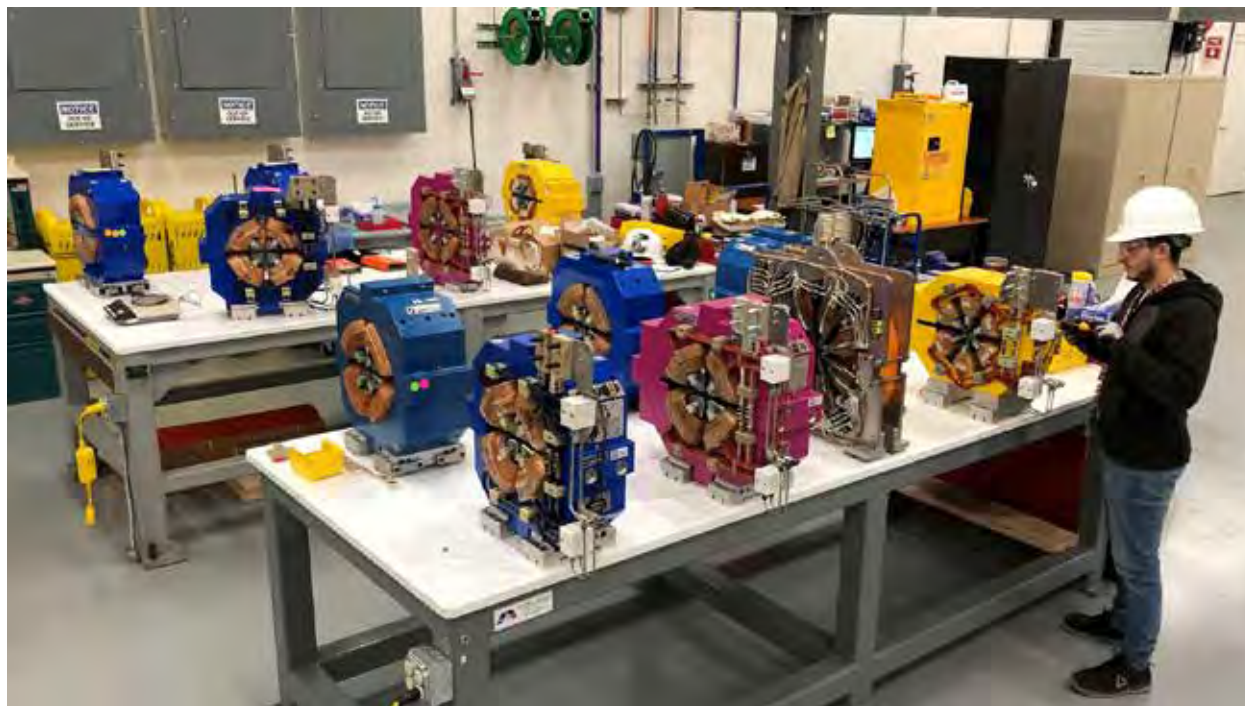
Fig. 3.4. Magnet measurement technician Gentillo Curescu works with an array of magnets for the Advanced Photon Source Upgrade construction project. A total of 1,321 magnets will be installed during the upgrade. [Courtesy Argonne National Laboratory]
