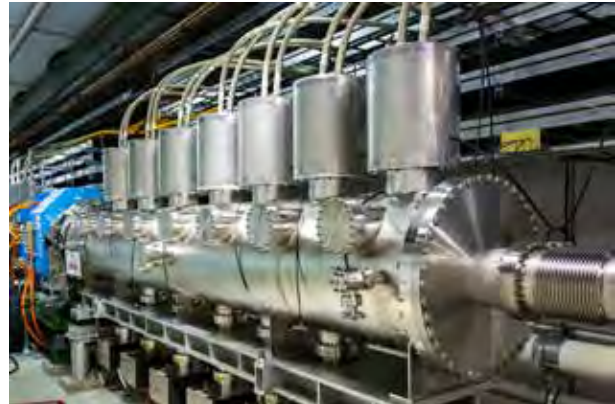
Fig. 3.8. Linear accelerator (linac) for the Spallation Neutron Source, which accelerates ions to very high energies. The linac is a superposition of normal conducting and superconducting radio-frequency cavities that accelerate the beam and a magnetic lattice that provides focusing and steering. [Courtesy Oak Ridge National Laboratory]
