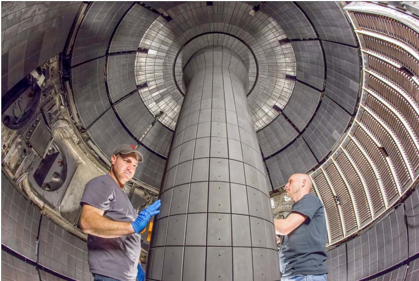
The newly installed center stack for Princeton's National Spherical Torus Experiment
