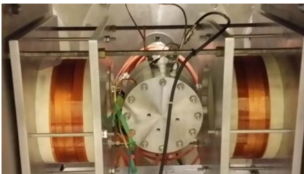
FIG. 3. Bench-test setup used for MGI valve testing in an external magnetic field. The valve is located between two external field coils.
