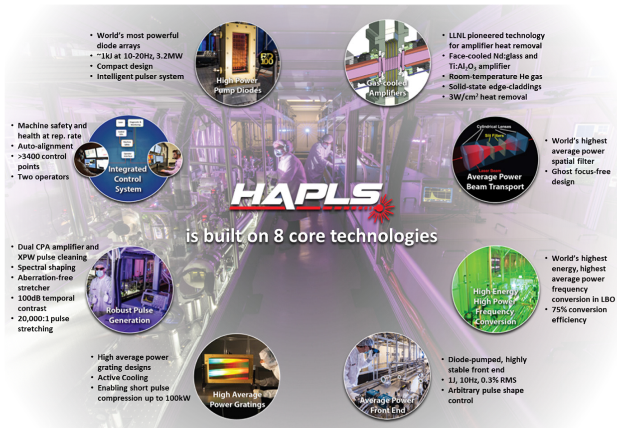
Figure 4.1: The High-Repetition-Rate Advanced Petawatt Laser System (HAPLS) architecture is based on eight major key laser technology leaps that enable high peak power pulses with 10Hz repetition rate.
