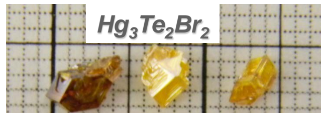
Single crystals of \text{Hg}_3\text{Te}_2\text{Br}_2 grown by vapor transport (grid is 1 mm)
