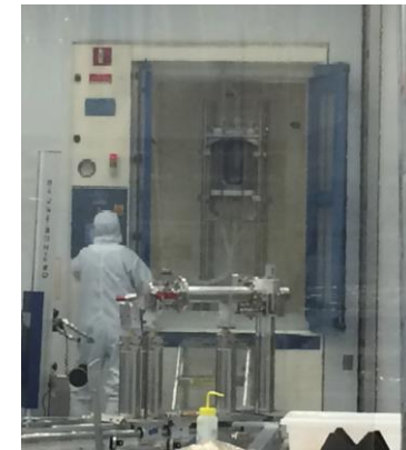
RF Dipole (RFD) chemical processing
