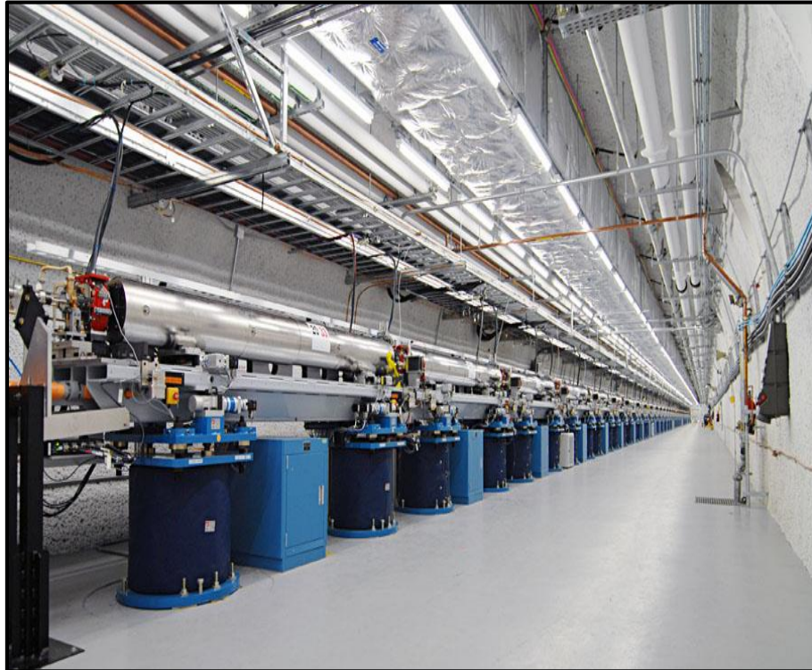
Shown is a portion of SLAC's two-mile-long linear accelerator (or linac), which provides the electron beam for the new Linac Coherent Light Source – the world's first hard x-ray, free-electron laser. For nearly 50 years, SLAC's linac had produced high-energy electrons for physics experiments. Now researchers use the very intense X-ray pulses (more than a billion times brighter than the most powerful existing sources) much like a high-speed camera to take stop-motion pictures of atoms and molecules in motion, examining fundamental processes on femtosecond timescales.
