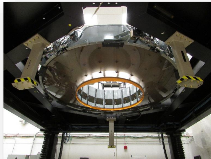
3.5m diam secondary mirror completed
