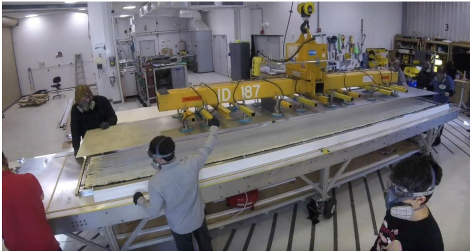
Cosmic Ray Veto Module Construction, University of Virginia
