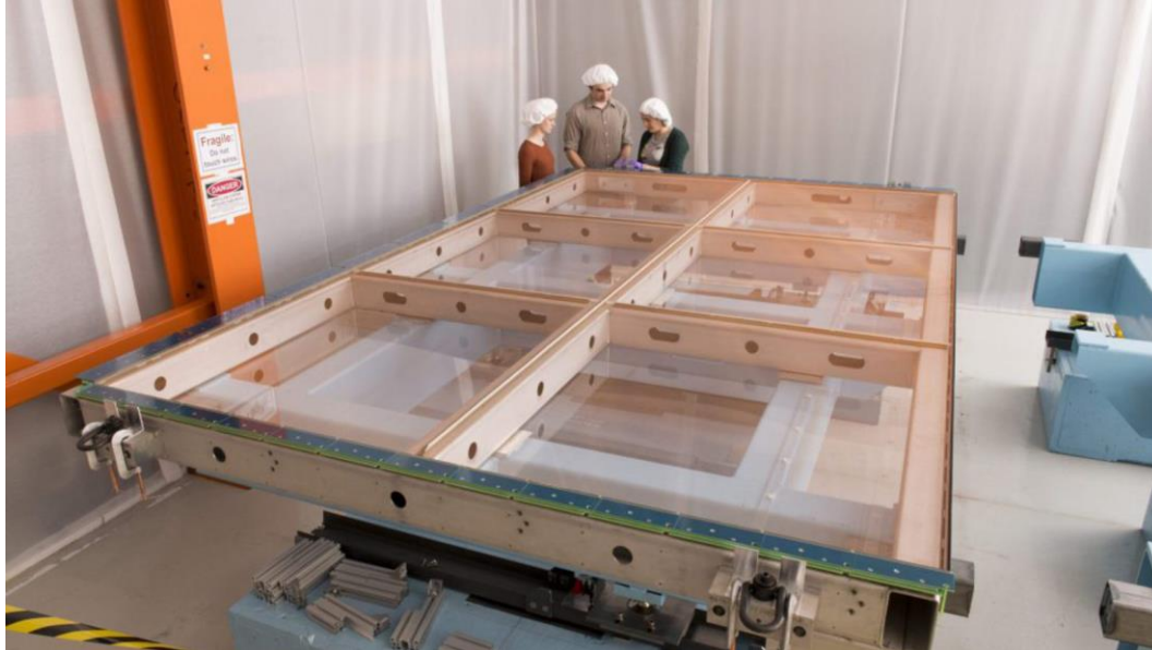
One of 4 wire planes (APA) in the SBND TPC (Fermilab)
