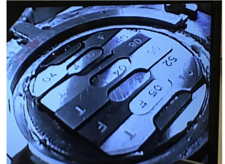
Tensile testing of Ti alloys at PNNL for targetry
