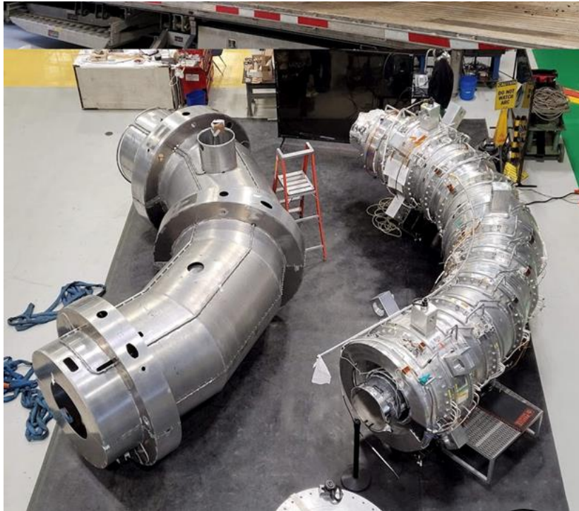
The TSu outer thermal shield was delivered to Fermilab in March (left). The thermal shield is a clam shell that will be installed around the outside of the TSu coldmass (right).
