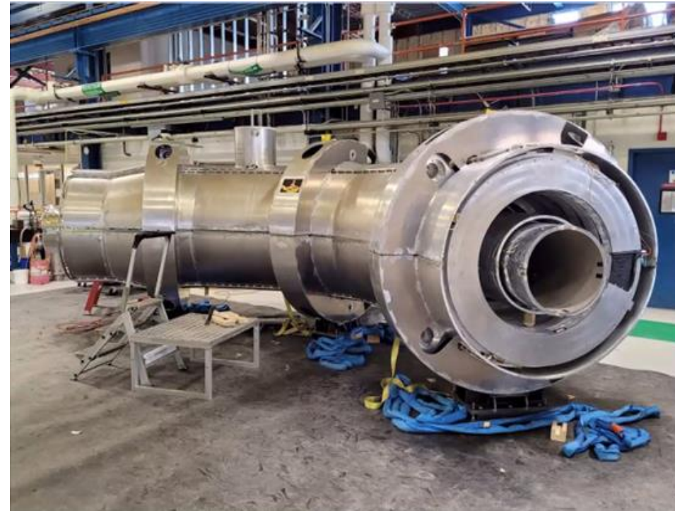
Dry fit of TSu outer thermal shield to look for interference issues. A few were identified and can be easily resolved.
