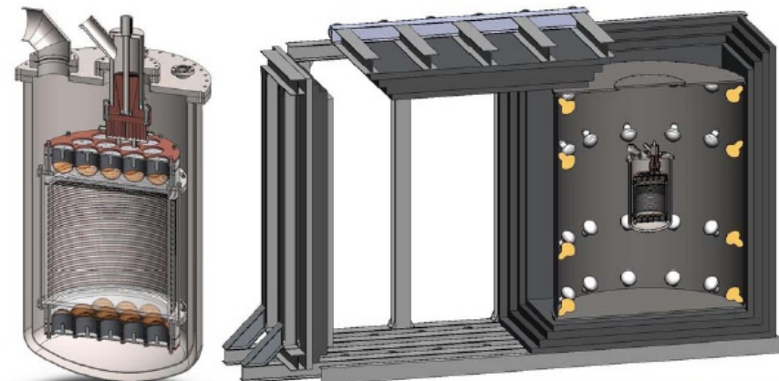
FIG. 5: (a) The DARKSIDE-50 internal detector. (b) The DARKSIDE-50 detector within the active liquid scintillator neutron veto and the passive shield.
