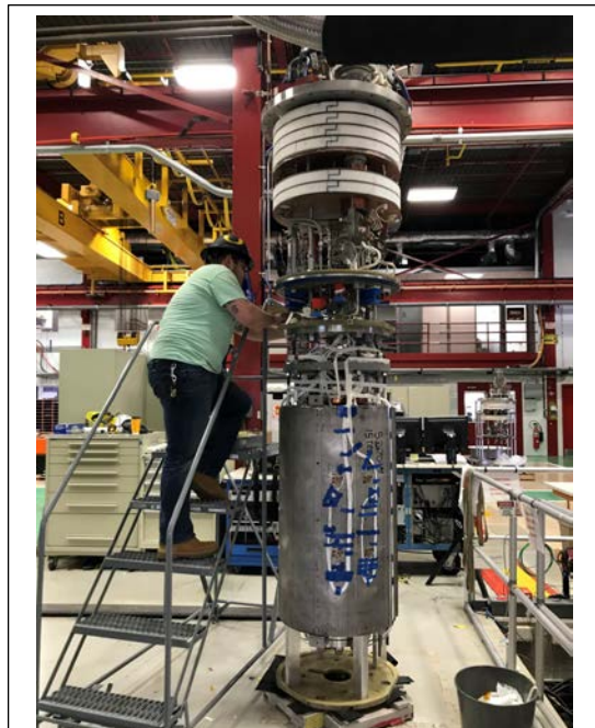
Figure 1. The 60-mm aperture dipole demonstrator MDPCT1 being prepared to cold tests. The magnet reached the record field of 14.5T in June 2020.
