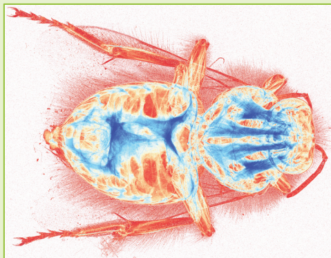
Color image of a bumblebee taken with Medipix3 on silicon, 55µm pitch, 7x8 tiles, 20kV / 100µA / Mag. 4x, Object height ~25mm. Image from the Ph.D. dissertation of Simon Procz, University of Freiburg.
