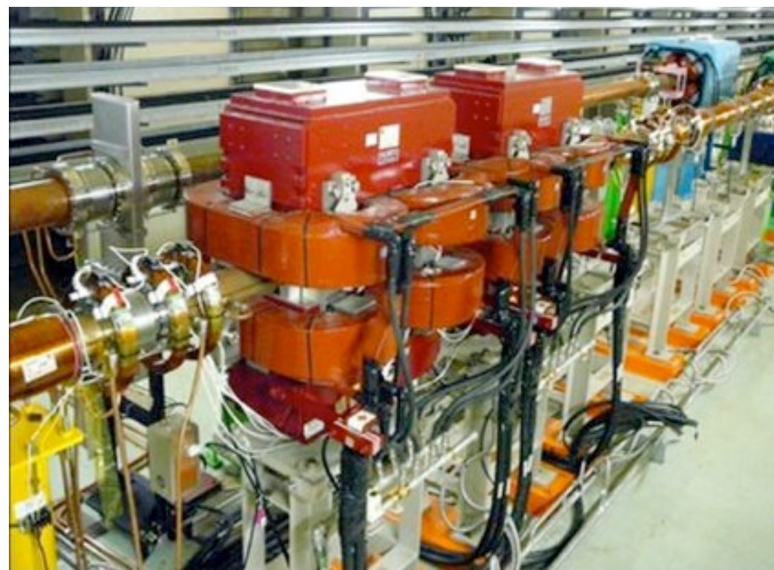
Wiggler magnets B = 0.77 \text{ T}
