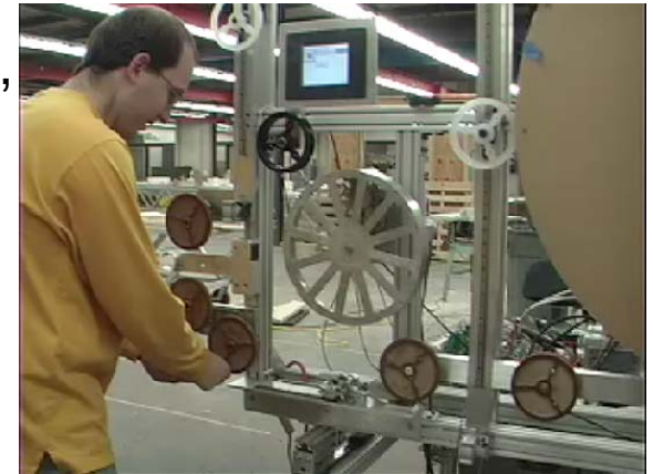
Fiber stringing machine at the Minnesota factory
