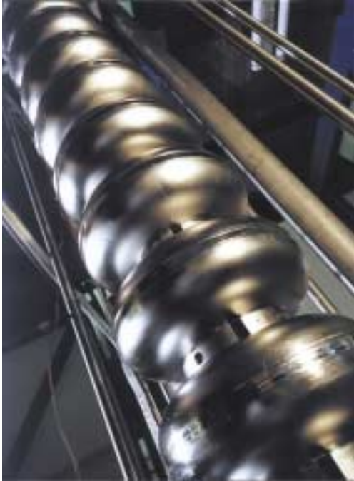
TESLA Superconducting Cavity
