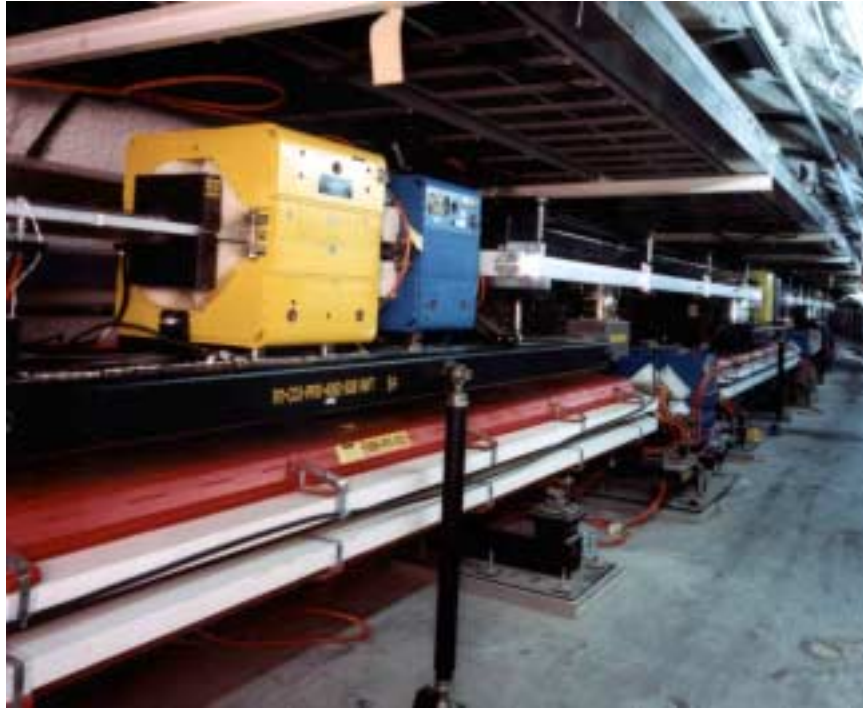
Figure 2.1. The PEP-II Accelerator at SLAC. PEP-II accelerates electrons (bottom ring) and positrons (top ring), colliding them in the BaBar detector.
