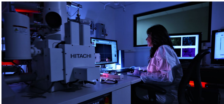
Scanning electron microscope used to characterize nano-antennas. (Credit: Savannah River National Laboratory)
