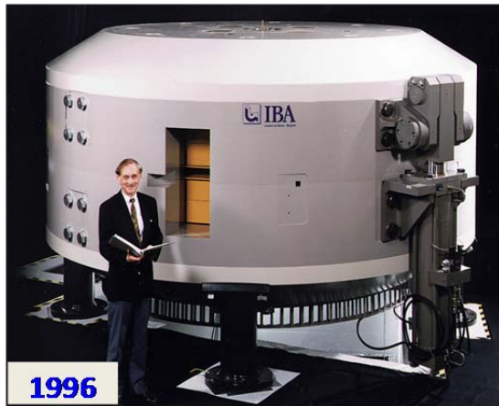
Figure IV-1. Comparison of 250 MeV proton therapy machines sold in 1996 (left) and 2012 (right). The latter, a superconducting synchrocyclotron made by MeVion Medical Systems, is small enough to be installed on a gantry system that rotates the accelerator around the patient. The new design shares some features with an isochronous superconducting cyclotron designed for neutron therapy a decade ago. Design features of the superconducting neutron and proton therapy machines can be traced to the NSCL. In this application size does matter, smaller is cheaper.
