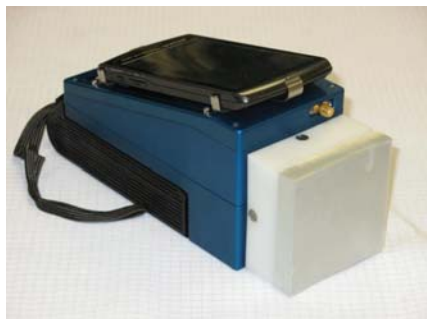
Figure IV-6. The prototype of a new type of hand-held survey meter developed by the Los Alamos National Lab that makes use of the inorganic scintillator CLYC and a pulse-shape-analysis signal-processing chip both developed for basic nuclear science research. CLYC stands for a crystal with the composition \text{Cs}_2\text{LiYCl}_6:\text{Ce} . The survey meter allows for isotope identification, directionality determination, and threat assessment.
