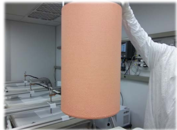
Inspection of copper being electroformed at the Temporary Clean Room in SURF
