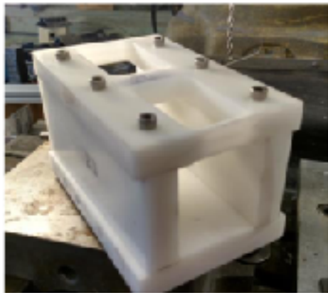
Mold for casting blocks
