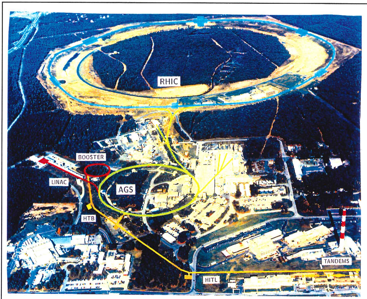
Aerial view of the Relativistic Heavy Ion Collider (RHIC) at Brookhaven National Laboratory. The existing Tandem van de Graaf accelerators, Booster Accelerator and the Alternating Gradient Synchrotron (AGS) will accelerate heavy nuclei for injection into RHIC. After further acceleration, two counter-rotating beams will collide at energies of up to 100 GeV per nucleon. The RHIC accelerator (3.8 kilometers in circumference) and associated experiments are under construction and expected to be completed for operation in 1999.
