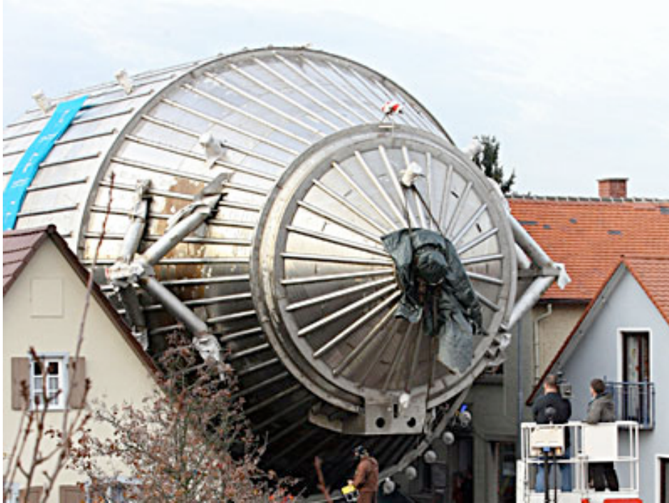
FIG. 4: The 10-m diameter tank for the KATRIN spectrometer moving through the town of Leopoldshafen on the Rhine, on its way to the Forschungszentrum Karlsruhe. The objective of the tritium beta decay experiment is a sensitivity to mass at the 200-meV level.
