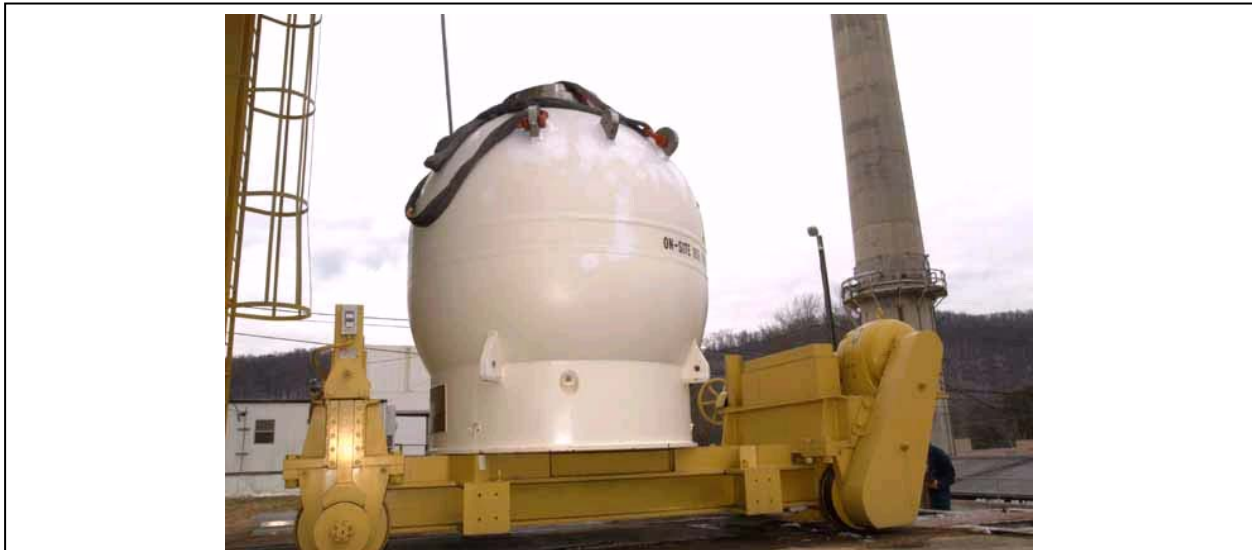
Figure 11.7: A SRP 25-ton Target Tube Cask Type B shipping container that is used for on-site shipments but has been decertified for off-site shipments.
