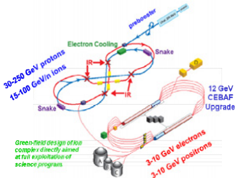
Figure 30. A schematic drawing for the Electron Light Ion Collider (ELIC) ring-ring concept. Image courtesy of Robert Ryne (Lawrence Berkeley National Laboratory).
