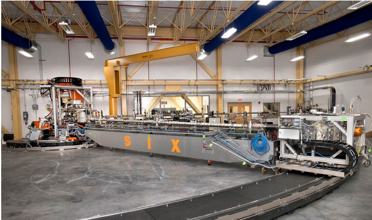
Fig. 2.3. At the National Synchrotron Light Source II, scientists use a technique called inelastic X-ray scattering to study the inner dynamics of materials and condensed matter. To achieve its extremely high energy resolution, the Soft Inelastic X-ray Scattering (SIX) beamline’s detector is positioned at the end of a long arm, which allows scientists to study samples from multiple angles. [Courtesy Brookhaven National Laboratory]
