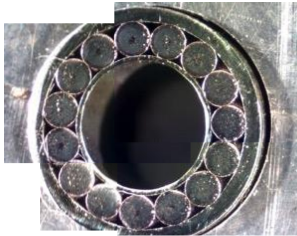
The cable is inserted in a sheath tube, and the sheath is drawn onto the cable to just compress the wires against the spring tube.
