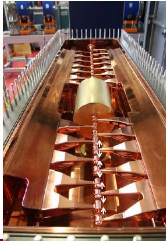
BNL EBIS Injector 100 MHz IH Structure (Courtesy of J. Alessi)
