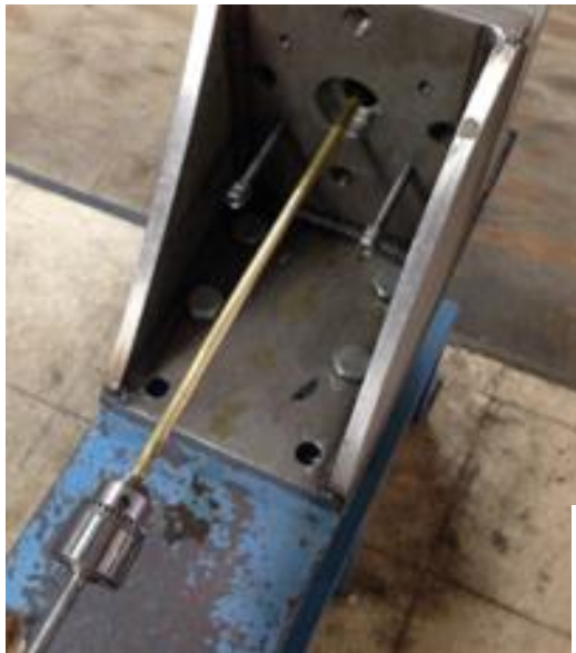
The cable is inserted in a sheath tube, and the sheath is drawn onto the cable to just compress the wires against the spring tube.
