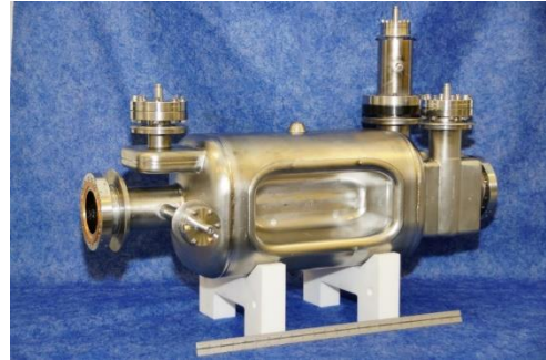
400 MHz prototype cavity for LHC with HOM couplers
