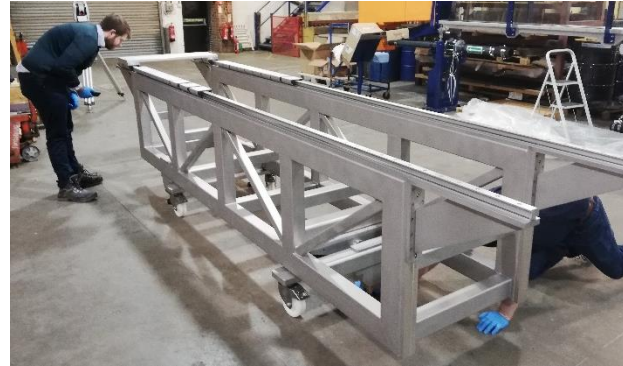
String assembly trolley
