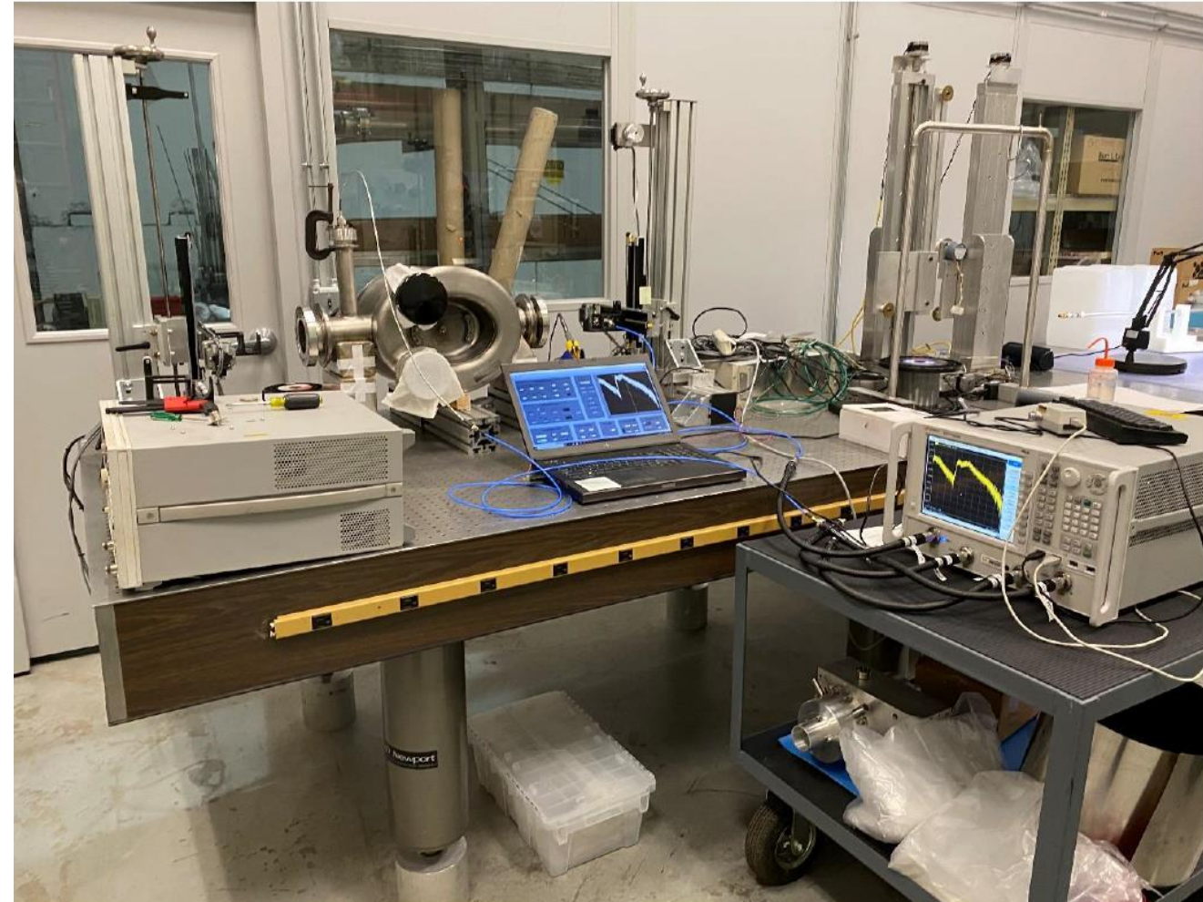
Stretched Wire System
