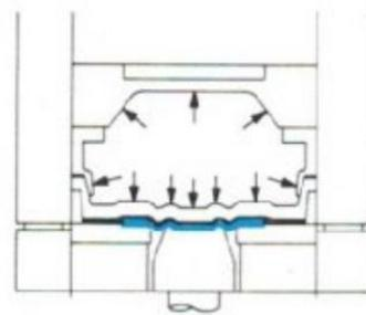
Forming Chamber is lowered and initial pressure is applied.
