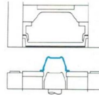
Pressure is released, forming chamber is raised, and punch is retracted from drawn part.
