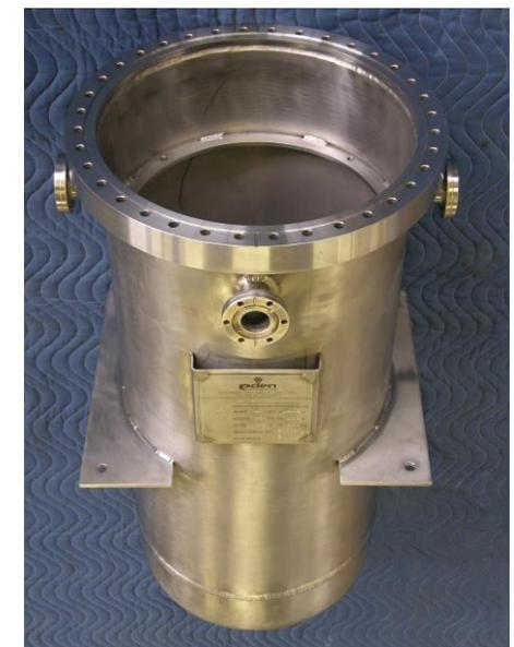
ASME U-stamped helium vessel built with collider funds 2010
