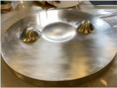
ANL-designed aluminum hydroforming dies
