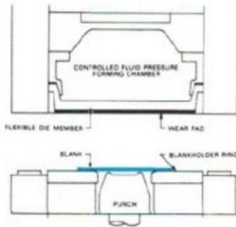
With forming chamber in raised position, blank is placed on blankholder ring.
