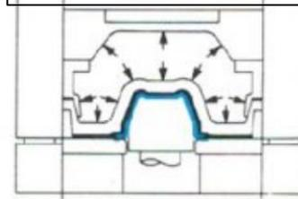
As punch moves upward, blank flows and wraps around punch.
