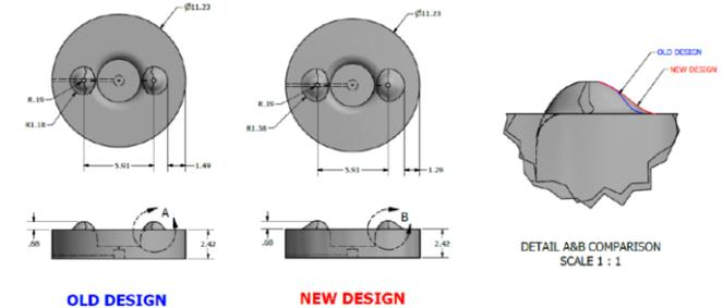
Figure 7: Step 3 forming. Note: the nub shown in the old design follows the profile of the nub used in the dome. The new design was adopted in the final toroid die.
