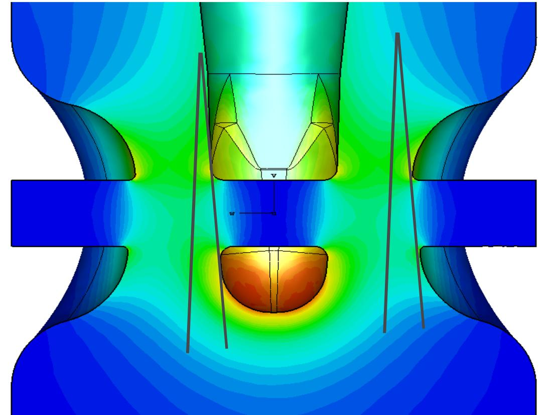
5 degree tilt on drift-tube faces produces transverse electric field that cancels on-axis magnetic field steering
