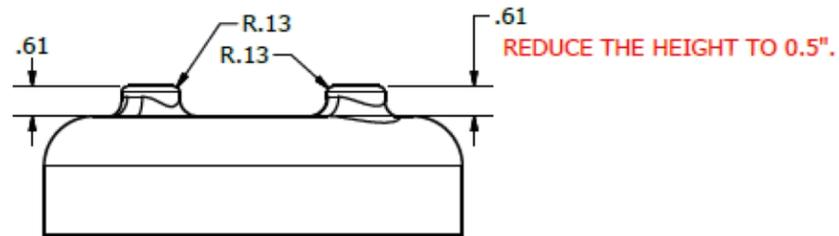
Figure 8: Step 4 forming. Note: the Al die was modified later at ANL Central Shops on 9/28/2021
