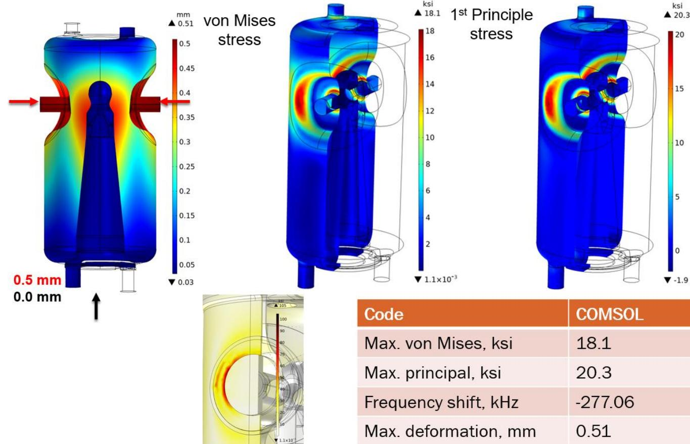
Stresses are tolerable and with a large useable tuning range
