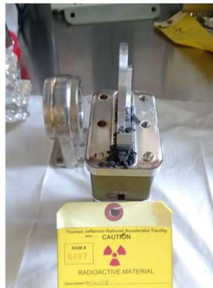
damaged beamline valve damaged magnet and cables
