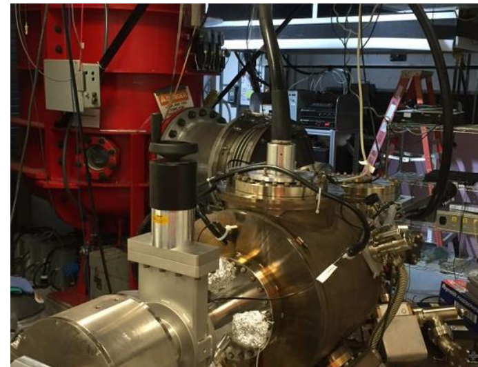
GTS 300 keV unpolarized load-lock photogun with inverted insulator
