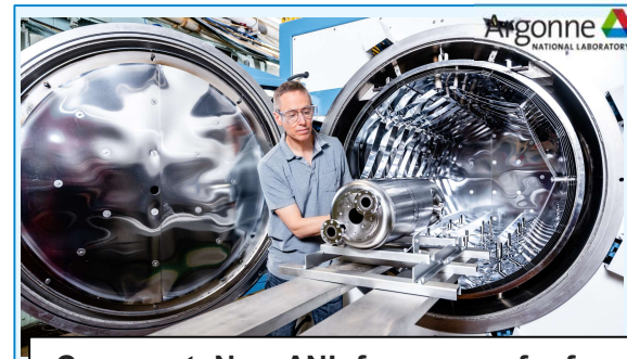
Comment: New ANL furnace so far for H 2 degassing → learning from FNAL, convert to Nb 3 Sn
