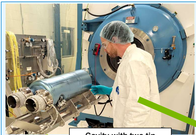
Cavity with two tin sources before coating
