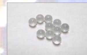
FB-CVD coated with Ti_{0.5}Si_{0.5}O_2
