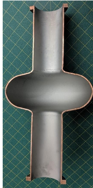
CVD Nb 3 Sn coating on CVD niobium interlayer on welded copper cavity substrate (Niowave)
