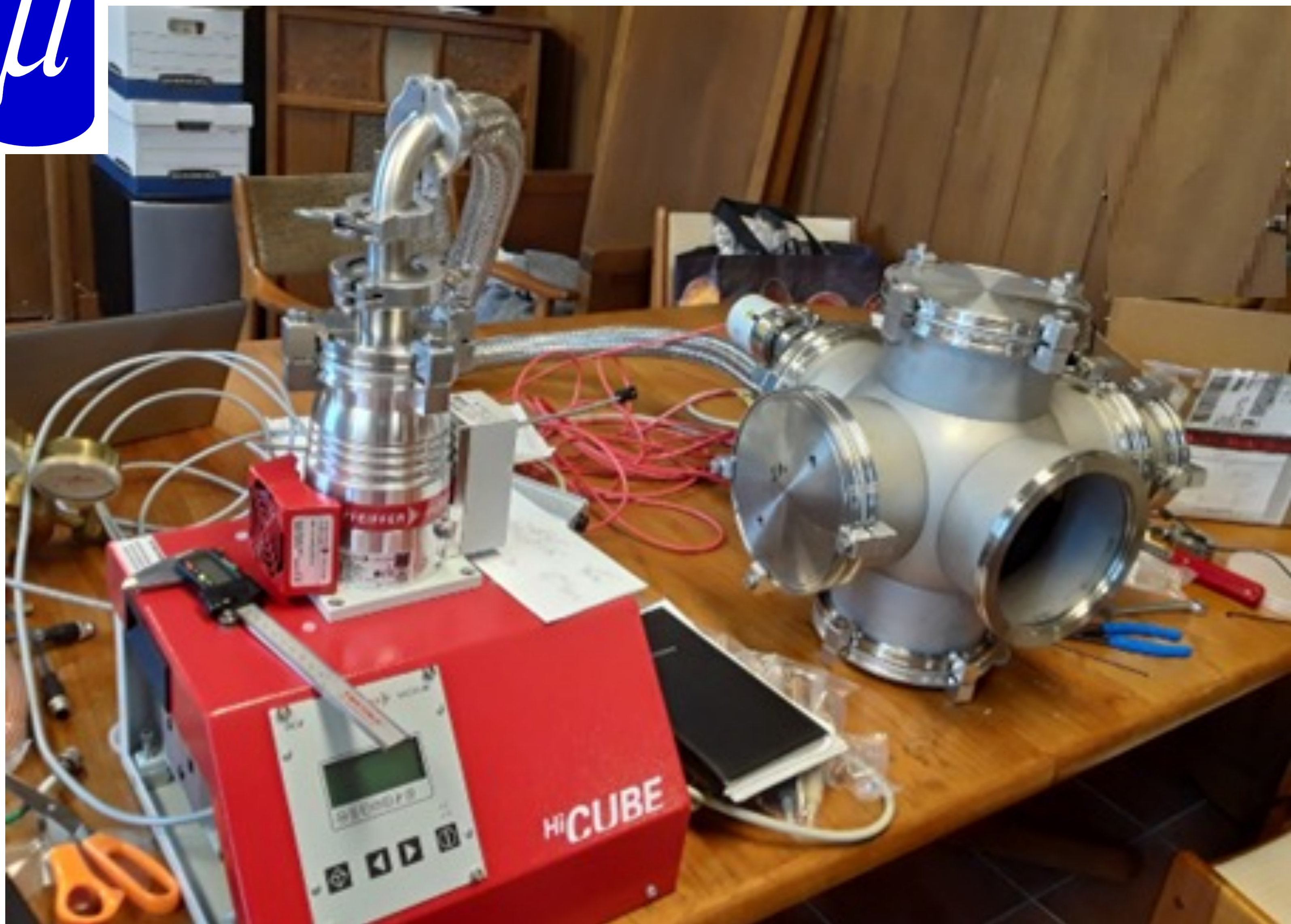
Fig.8. 6 - way cross with turbo pump.
