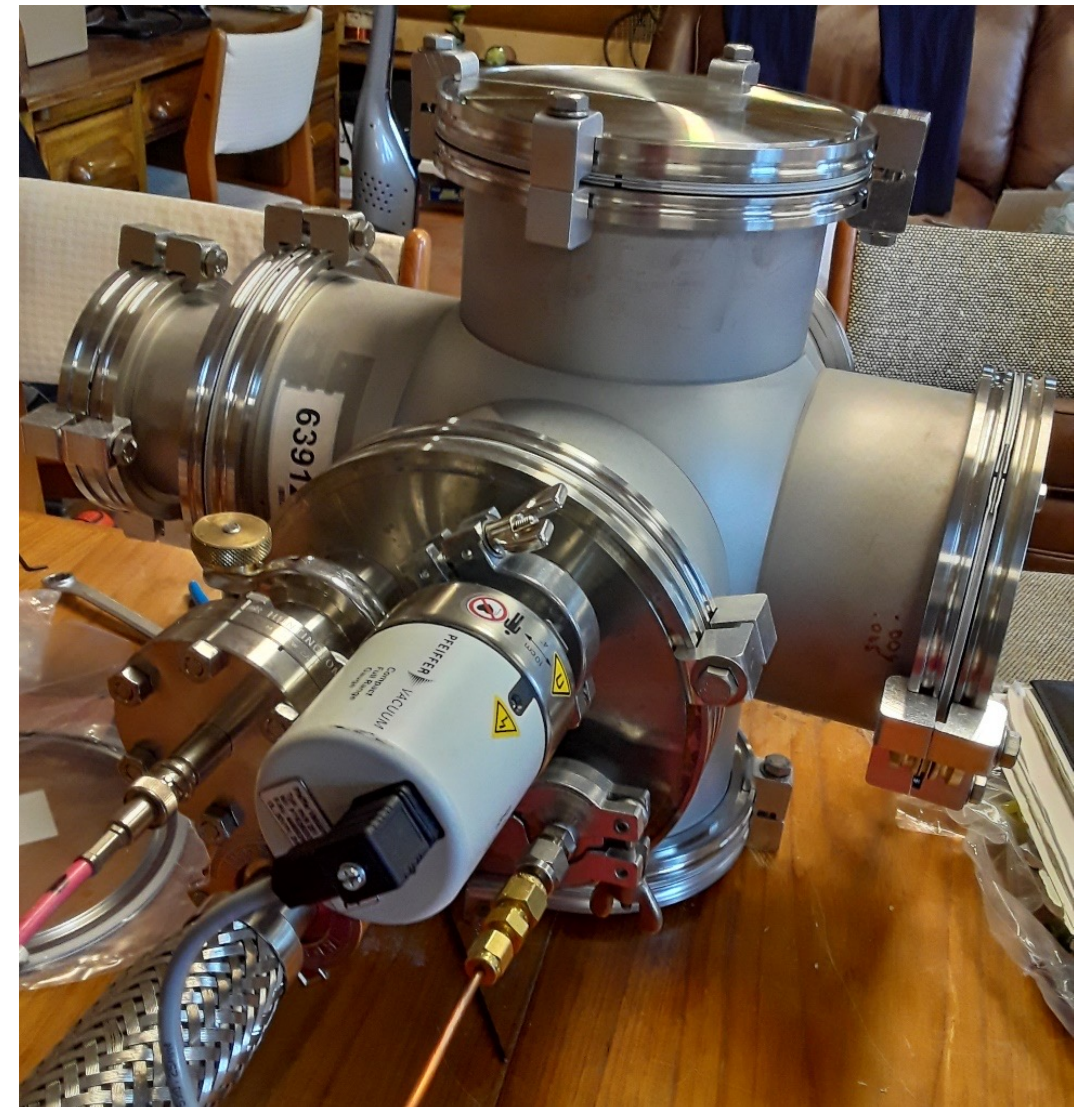
6-way cross with vacuum gauge and feedthroughs.
