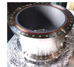
BNL LDRD three high power 308mm ID BLAs Technology: Shrink fit SiC (Coorstek SC-35)
