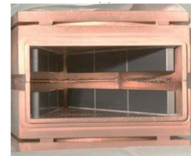
Argonne - APS WR284 Waveguide loads for SPX CM Technology: Soldering + EBW (St Gobain Hexoloy)
