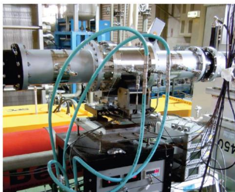
18kW high power tests of SiC at KEK in collaboration with Toshiba Energy Systems Technology: SiC
