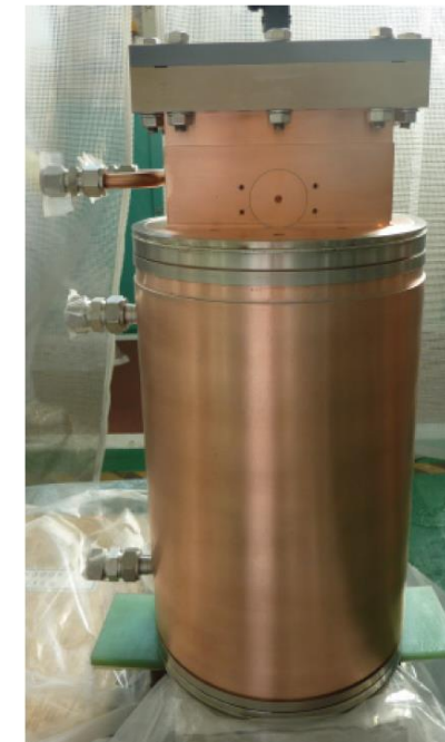
10kW, 1.428GHz Toshiba + KEK CERASIC from Covalent Materials Corporation
