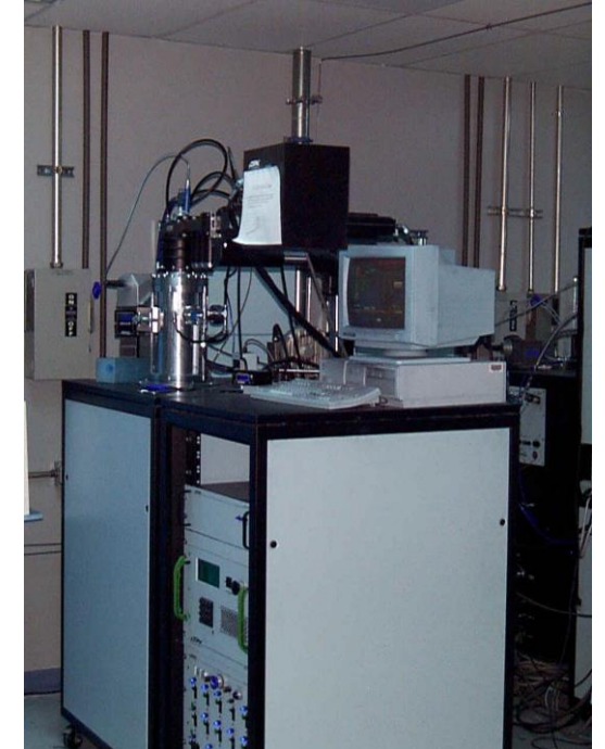
ASTeX PDS-17 microwave plasma enhanced chemical vapor deposition system
