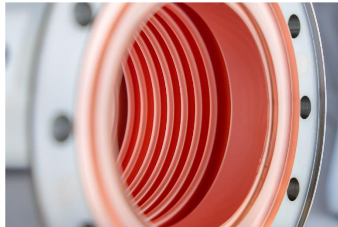
(Left) Photographs of a Cu-coated LCLS-II bellows section, which is presently being evaluated at JLab . (Right) Photographs of a Cu-coated edge-welded bellows.
