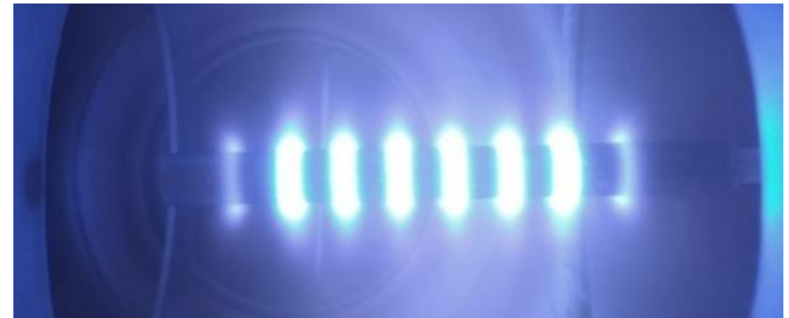
The prototype 0.5"-OD magnetron, which was made with an aluminum target.
