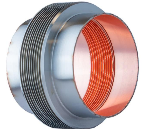
(Left) Photographs of a Cu-coated LCLS-II bellows section, which is presently being evaluated at JLab . (Right) Photographs of a Cu-coated edge-welded bellows.
