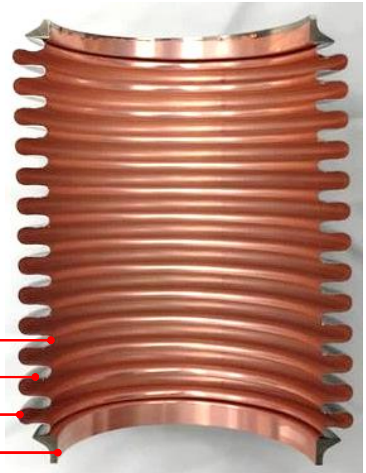
A cross sectioned piece of a Cu-coated bellows (right). The apparent delamination at the top is where Cu was intentionally peeled off for RRR measurements. Measurements of the RRR for two processes (made at the indicated locations) are given here as well (left)
