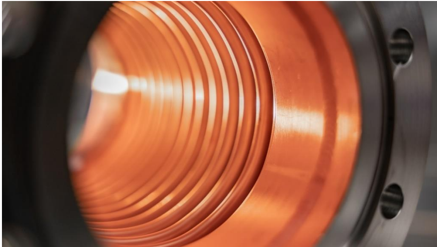
A Cu-coated bellows.
