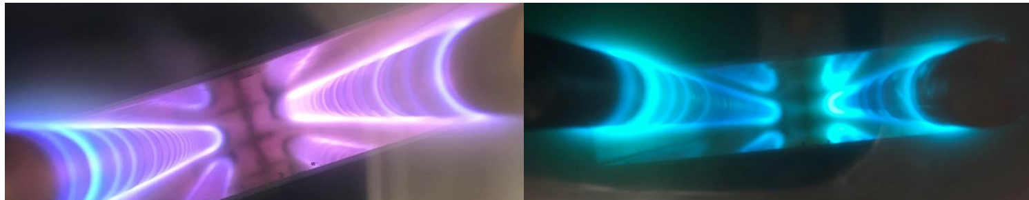
Photographs of the dual-magnetron configuration in-operation during the plasma-etch step (left) and main deposition step (right), taken with the top of the test fixture removed.
