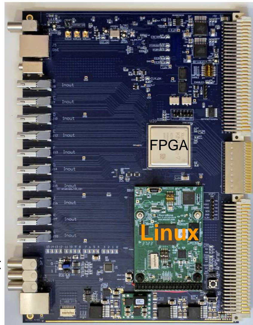
Logic & Trigger Module Serving 320 Channels
