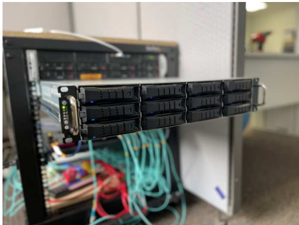
Data Collector servers receive event streams and convert them to files
