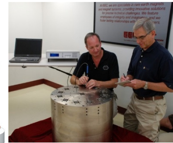
NIST Watt Balance PM assembly ~ 1800 lb.
