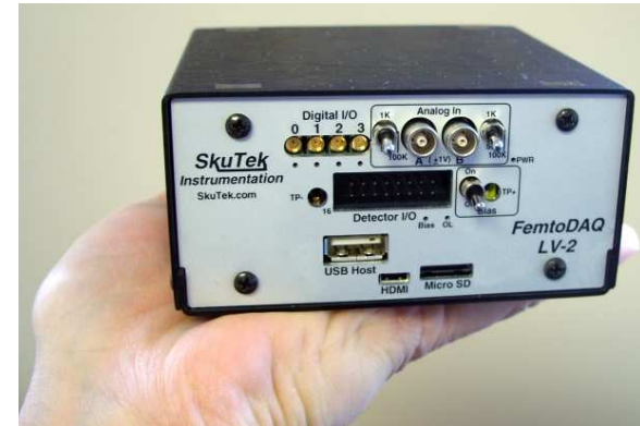
Low cost networked digitizer (2 channels)
