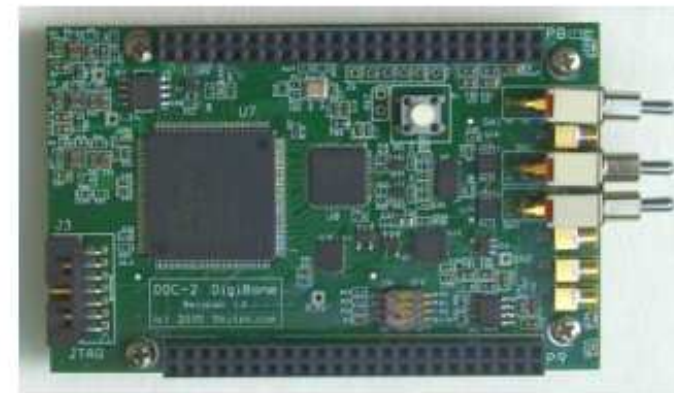
2-channel Digitizer: 14 bits, 100 MHz
