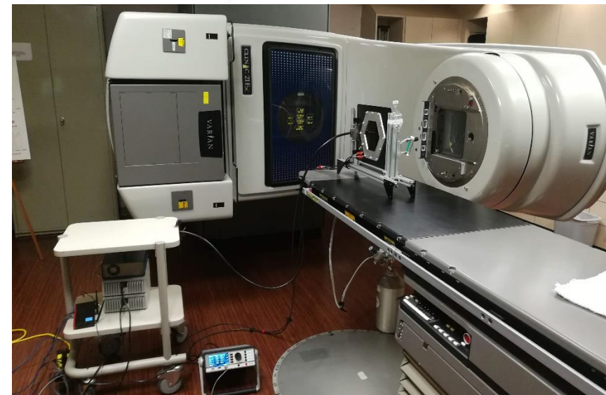
A set-up of the technology tester detector in an x-ray beam
