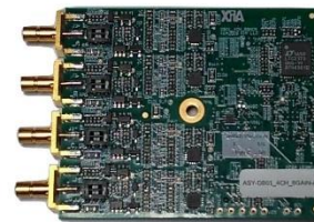
4-channel, 75-125 MHz, 14bit ADC daughter card
