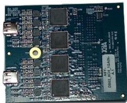
8-channel, 250 MHz, 12bit ADC daughter card Differential inputs via HDMI cable
