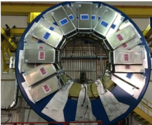
Inside face of east pole-tip, partially installed
