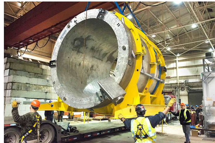
The solenoid magnet that will form the core of the sPHENIX detector
