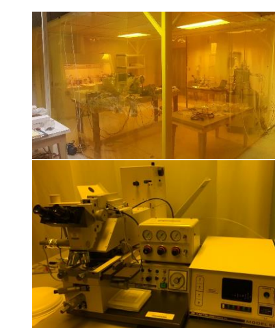
Figure 11. The photolithography and metallization equipment installed in the new clean room (above), Karl Suss MJB-3 mask aligner with 365-405 nm 300 W UV Hg-lamp (below).
