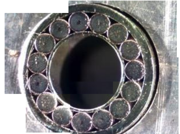
Cross section showing NbTi strands
