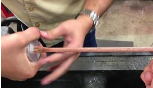
cabling wires onto perforated spring tube
